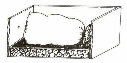
Fig. 1. Cross section of the styropore box used for storing mussel in ice.
